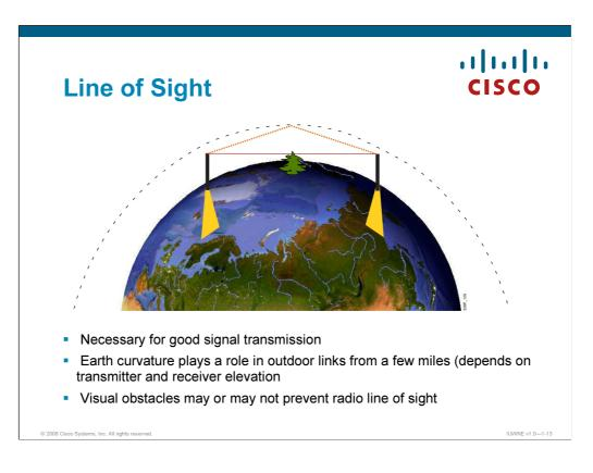
As a signal travels in a straight line towards a receiver, it will be received in good condition if there is clear line of sight between the sender and the receiver. If there is an object in the path of the wave, such as a tree or a building, then the attenuation (absorption) and other phenomena will prevent communications from occurring.
