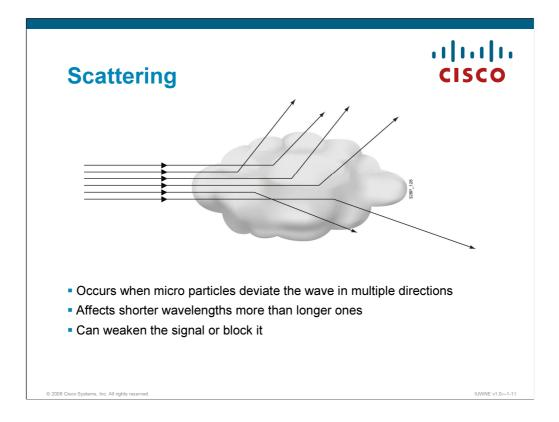
Reflection relates to major obstacles, but it also occurs in the air itself. If the radio wave and the air particles could be seen, it would show that some of them, such as dust or micro drops of water (humidity), would affect the wave. These multiple reflections are described as **Scattering**.
