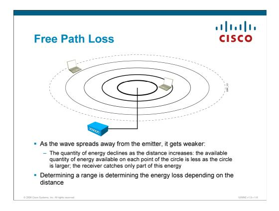
A radio wave emitted by an access point will be radiated in the air. If the antenna is said to be omnidirectional, the signal will be emitted in all directions, just like when throwing a stone in water, waves radiate in all directions from the point where the stone touched the water. If the antenna is directional, the beam will be more focused.
