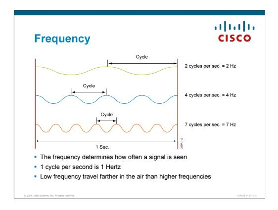
The wave is always sent at the speed of light as it is a magnetic field. This means that it will take a shorter or longer time to travel one cycle: if a signal wavelength is 5 millimeters long, it will take less time to travel a cycle than if it is 400 meters long, as the speed is the same in both cases. The natural consequence of this difference will be that, as the longer signal takes more time to travel one cycle, there will be less of its cycles in one second than of the first one.
