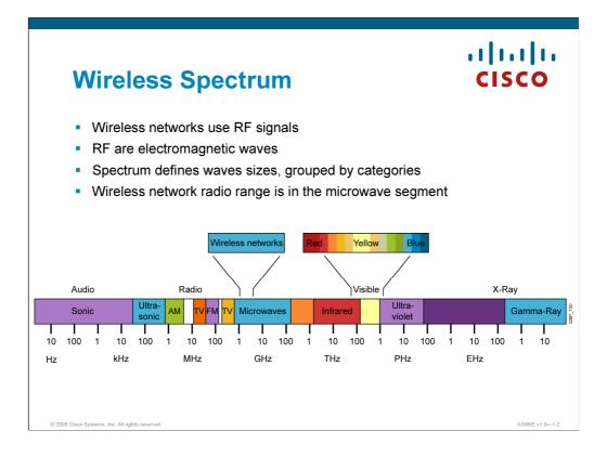
Many devices use radio waves to send information. A radio wave can be defined as an electromagnetic field radiated from a sender. It propagates to a receiver that receives its energy. Light is an example of electromagnetic energy. The eye can interpret it to send its energy to the brain, which will in turn transform it into impressions of colors.
