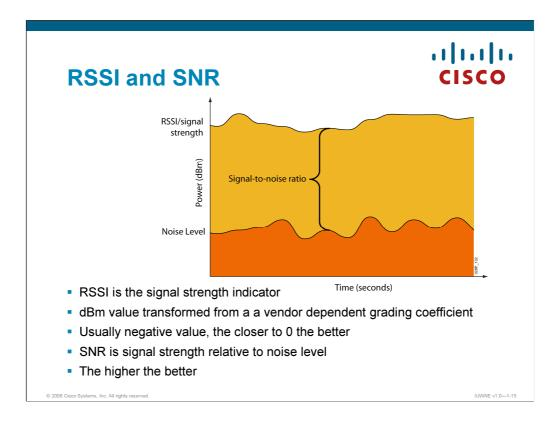
As the RF wave may have been affected by obstacles in its path, it is important to determine how much signal will be received by the other endpoint. If sender and receiver are compatible devices (e.g. two bridges, or an access point and a client WLAN adapter) the signal will probably not be too strong but it can be too weak to be heard or detected as an actual signal by the receiver.
