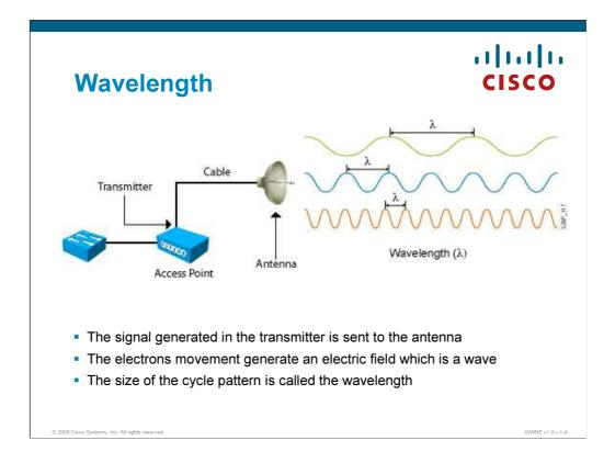
An RF signal starts with an electrical alternating current (AC) signal generated by a transmitter. This signal is sent through a cable to an antenna where it will be "radiated" in the form of an electromagnetic wireless signal. Changes of electron flow in an antenna, otherwise known as current, produce changes in the **electromagnetic fields** around the antenna and transmit **electric and magnetic fields**.
