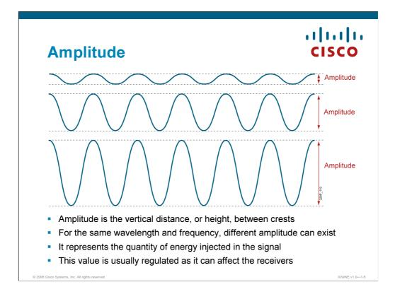
Another important factor affecting how a wave is sent is **amplitude**. Amplitude can be defined as the strength of the signal. From a graphical perspective, it is represented as the distance between the higher and lower crest of the cycle.
