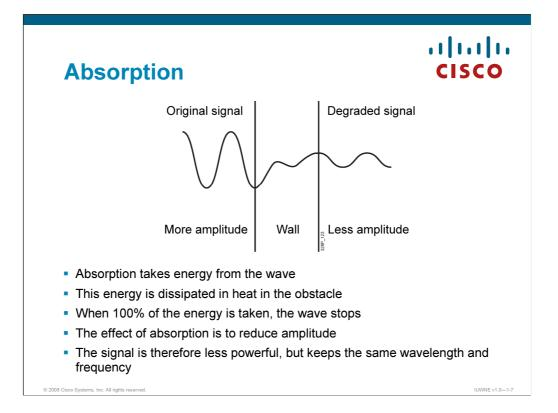
As the signal travels away from the access point, it will lose energy not only as free path loss but even more as passing through different types of material. Each material will take part of the energy just like the copper cable. In the air, dust and humidity (water drops) will be warmed up by the signal, thus weakening it.
