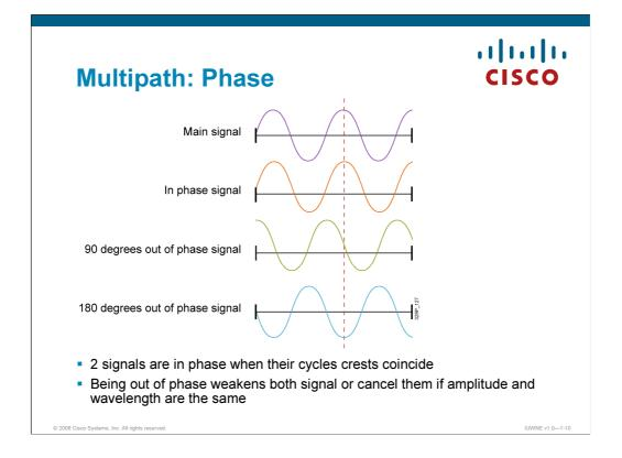
But if both signals are not sent at exactly the same time, the receiver may get the first positive crest, then as it receives the first subsequent negative crest, it may receive the second positive crest, receiving a positive signal to which the same exact negative signal is added results in a neutral signal, or no signal at all.
